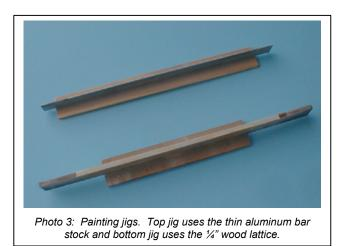
thinner vertical piece is needed when airbrushing the 1:6000 models. For this scale (and some of the smaller fleet units in the larger scales), I use a piece of 1/16" aluminum flat bar (1" wide) attached to a wood lattice base. You'll have to cut a lengthwise slot in the wood base before gluing the aluminum bar to it with epoxy or construction adhesive. Again, a thin strip of heavy-duty carpet tape is used to hold the models in place while painting.
