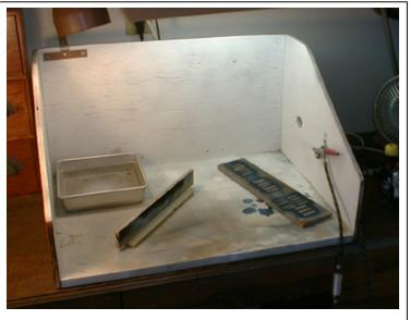
Photo 1: A simple plywood spray booth for airbrushing.
